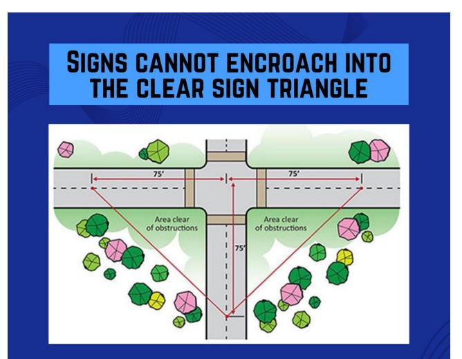
The clear sight triangle is the area between curb lines of an intersection and line connecting points at a specific distance from the corner of the intersection and such corner is determined by projecting the curb lines out to a specific point
