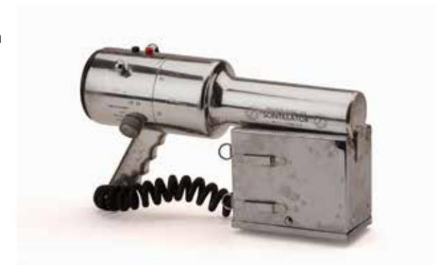
customers are informed that owners of small planes can earn up to \$30 an hour plus a percentage of claims while surveying with a scintillator. Using this scintillator, which looks like a chrome-plated ray gun from a 1940s science fiction thriller, prospectors set out with hopes of striking it rich.
