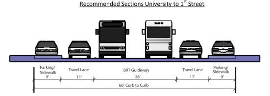
The Central Avenue cross-section would continue to have two travel lanes in each direction. From University to Broadway the roadway would be widened throughout to create the exclusive lane during peak hours. During off-peak hours, the BRT could operate in the current outside lane and enter queue-jumper lanes around signalized intersections. On-street parking would be allowed away from signalized intersections.
