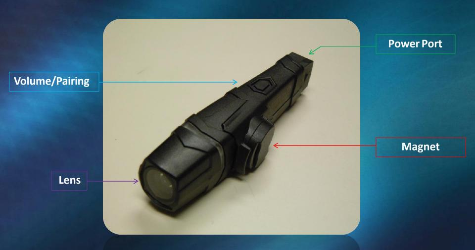
All video and audio footage is stored in the Camera. The Battery Pack only contains the power source and the controls.
