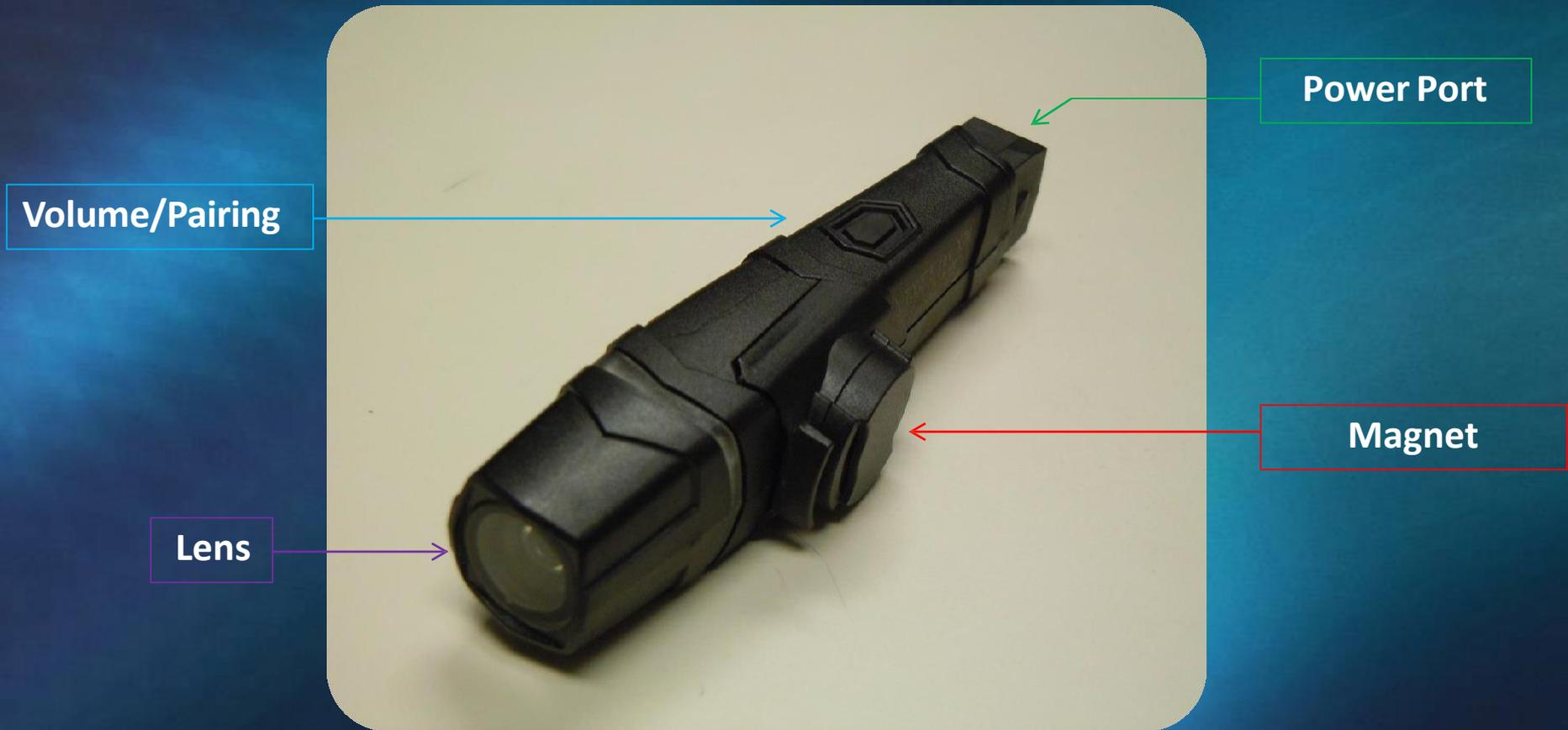
All video and audio footage is stored in the Camera. The Battery Pack only contains the power source and the controls.
