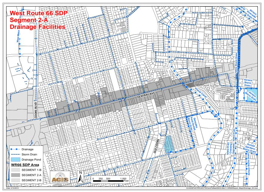
Figure 34: Drainage Facilities, Segment 2-A
