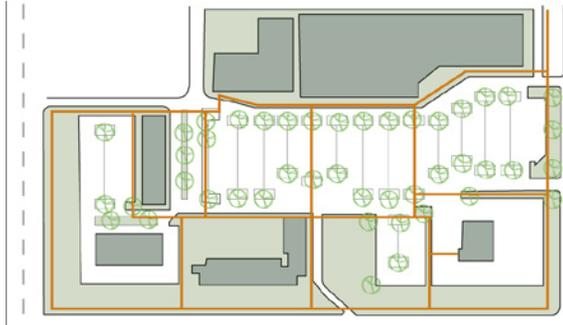
Plan diagram showing pad site development with internal bays of parking, clear pedestrian access (orange lines) and street edge definition.
