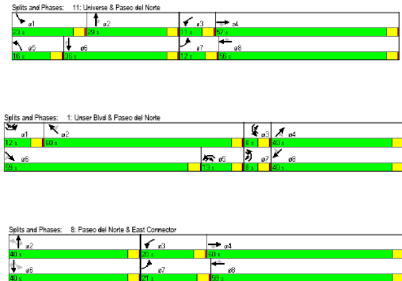
Figure 2-7 Signal Timing Concept: Planned Intersections
