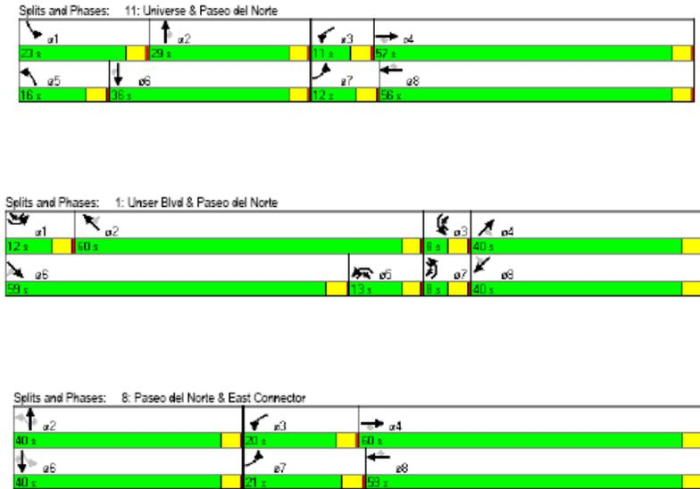
Figure 2-8 Signal Timing Concept: Proposed Additional VHSDP Intersections on Paseo del Norte
