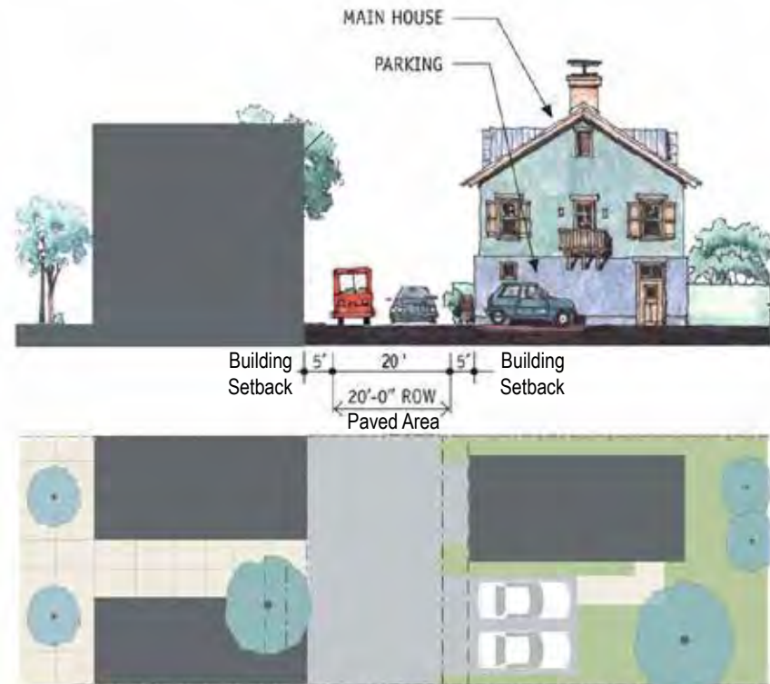
Exhibit 10.23 – Typical Commercial Alley Cross Section
