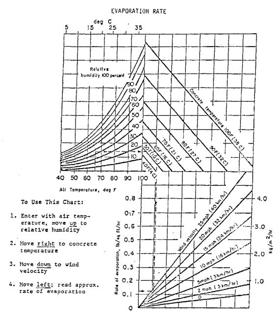
Effect of concrete and air temperatures, relative humidity, and wind velocity on the rate of evaporation of surface moisture from concrete. This chart provides a graphic method of estimating the loss of surface moisture for various weather conditions. To use the chart, follow the four steps outlined above. If the rate of evaporation approaches 0.2 lb per sq ft per hr (1.0 kg/m<sup>2</sup>/hr), precautions against plastic shrinkage cracking are necessary.
