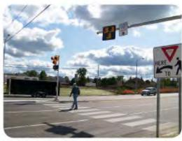
Pedestrian hybrid signal; also called HAWK signals (High-Intensity Activated Crosswalk).
