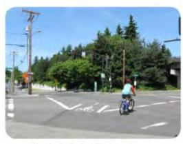
Scramble signals allow cyclists to cross a intersection diagonally.
