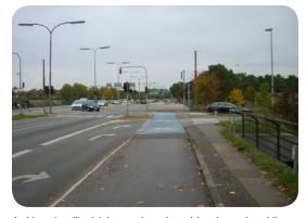
At this unsignallized right turn, the cycle track has dropped to a bike lane with blue coloration and pavement markings through the conflict area.
