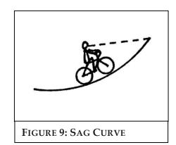
In general, vertical curve grade transitions should be designed to provide as gentle a transition as possible, given the physical constraints of a site. The table below provides suggested lengths of vertical curves for various conditions, based on 2% increments in grade change. These numbers are generalized and should provide acceptable results in most cases; however, if more detailed information is required, please refer to the current AASHTO Guide.
