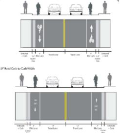
Two Lane Cross-Section with No Parking\*. \*Bike lanes may be 4' in width under constrained circumstances.
