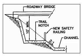
FIGURE 12: DEPRESSED UNDERPASS FOR LOW BRIDGE CLEARANCE CONDITION
