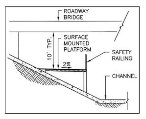
One of the primary concerns about placing trail crossings within major drainage channels lies in the fact that users are essentially directed into a potentially dangerous situation, where storm runoff may inundate the trail. Although the probability of such an occurrence would be quite low at any given time, it is nonetheless a valid concern. The safety of such a crossing can be greatly increased through the following actions:
