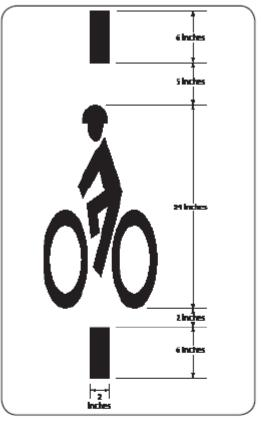
Recommended loop detector marking design.
