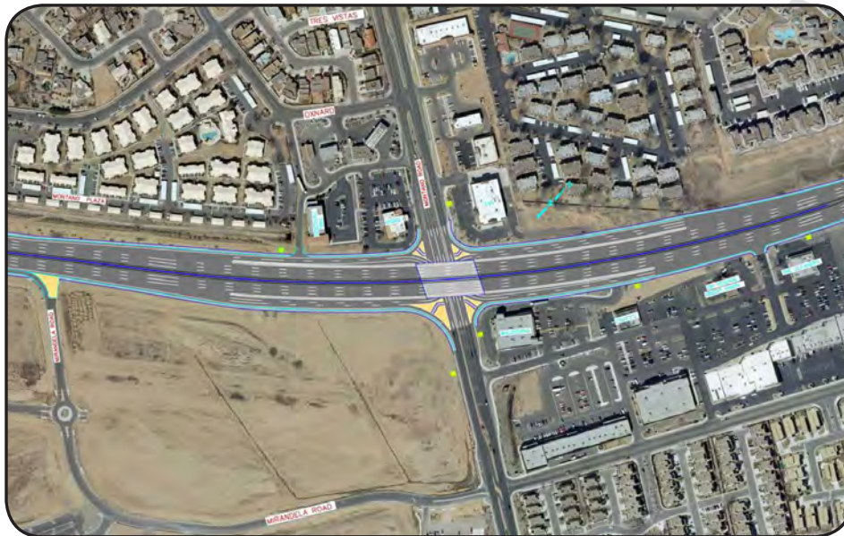
Figure C-7: Conceptual Single-point Diamond Interchange at Montañero Road
