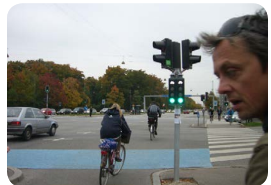
Bike-specific signals are small and placed on the near-side of traffic.
