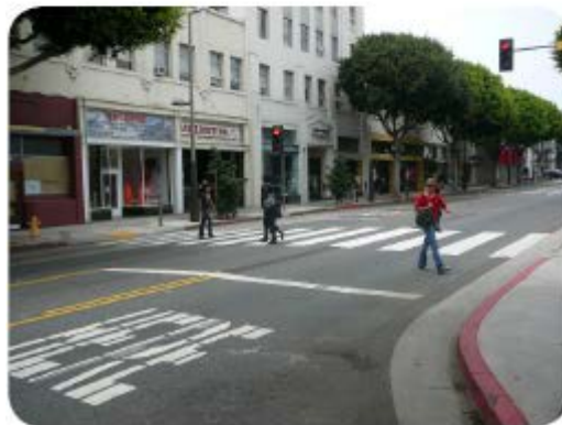
Advance stop bars alert motorists of pedestrians.
