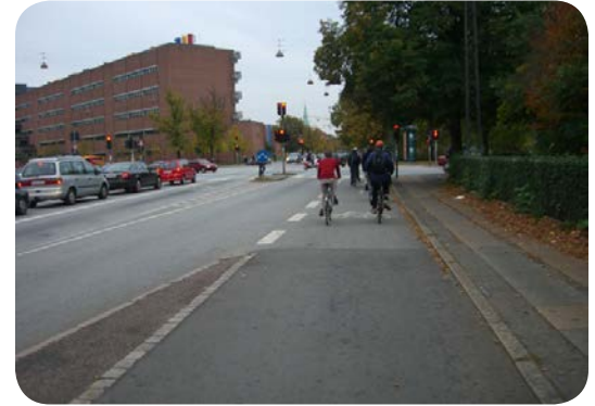
Cycle track dropping to bike lane before an intersection.
