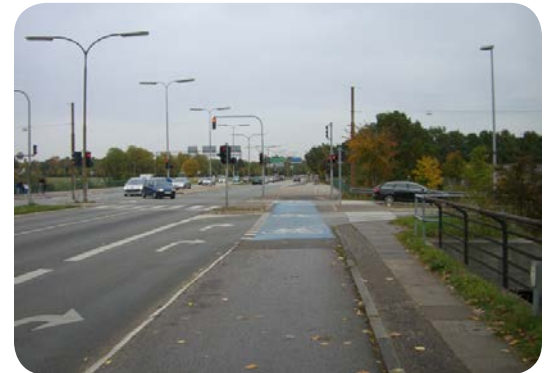
At this unsignallized right turn, the cycle track has dropped to a bike lane with blue coloration and pavement markings through the conflict area.
