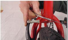
Using a wrench (15mm is standard) loosen axle nut on both sides of axle.
