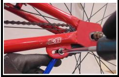
Place chain on teeth of front and rear cogs. Chain should still hang loose between cogs.
