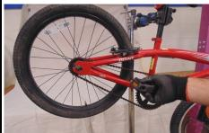
Reconnect hand brakes and/or tighten coaster brake arm bolt. Test brakes for effectiveness.
