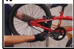
Tighten right (drive) nut. Test chain tension by pedaling back-
