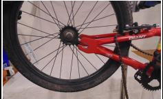
Once repair is complete, return wheel to dropouts. Ensure cog is on right (drive) side of bike.
