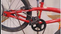
If hub has a coaster brake, loosely reattach brake arm.
