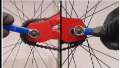
Allow the wheel to slide forward in the dropout. Remove chain from rear cog and hang on frame.
