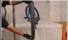
Pedal bike to test for brake rub, shift through gears to ensure all components are aligned.
