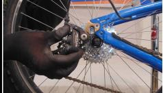
Once repair is complete, return wheel to frame. Ensure cog is on right (drive) side of bike.
