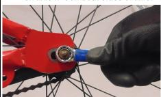
If wheel is a quick release, open cam lever on skewer.
