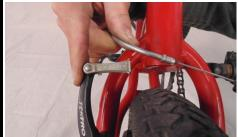
If bike uses cantilever brakes, connect straddle cable to non-bolted brake arm.
