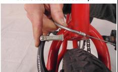
If bike uses cantilever brakes, disconnect straddle cable on non-bolted brake arm.
