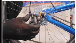
Tighten axle nuts/close quick release. Quick release should require some force to close.
