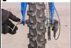
Pivot rear derailleur toward back of bike, allow wheel to drop down and remove from bike.
