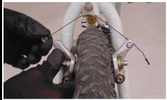
If wheel is bolted on, use a wrench (15mm is standard) loosen axle nut on both sides of axle.
