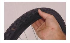
Install tube into tire, beginning with valve.
