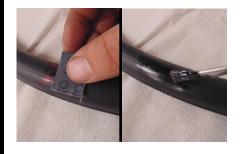
Once glue has set for five minutes, remove foil from patch and apply to puncture.
