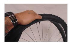
Starting near valve, push entire tire bead into rim channel.
