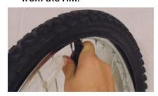
Completely remove tube from tire.
