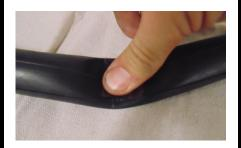
Carefully inspect inside of tire for sharp objects.
