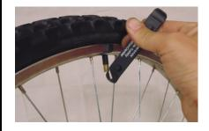
Use a tire lever to remove one side of the tire bead from the rim.
