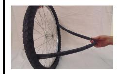
Inflate the tube and locate puncture. Mark location.
