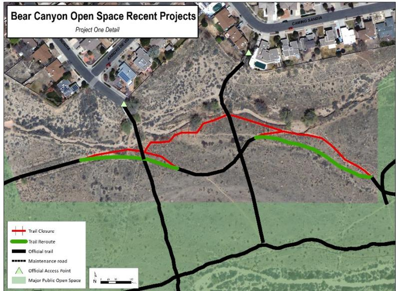
work on the private open space north of Bear Canyon West during October 2018 and July 2019, closing an eroding trail near incised drainage and formalizing a lower trail to form a connection across the private open space.
