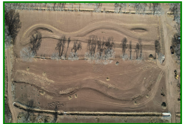
Fields 2B (top) and 2C (bottom) after construction of water conveyance slope and arroyo channel.
