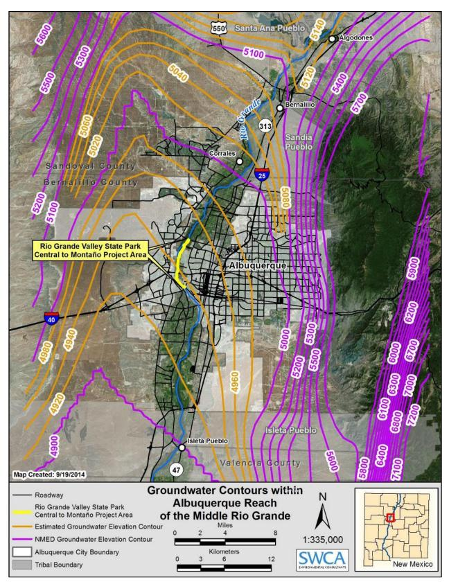
Figure 3.2. Estimated groundwater elevation.
