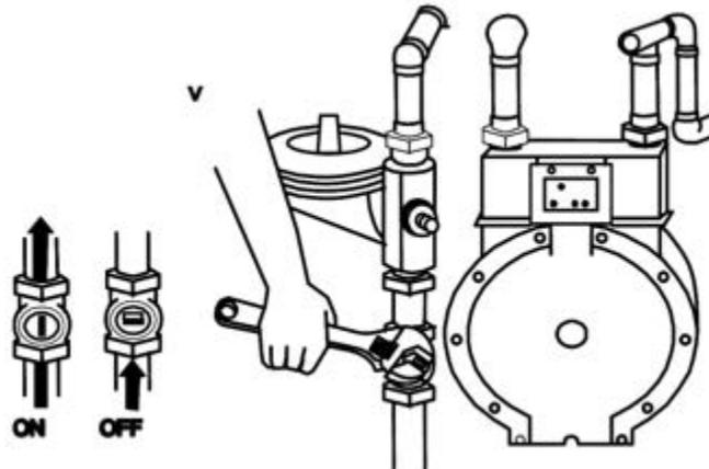
The gas meter shutoff diagram indicates the shutoff valve location on the pipe that comes out of the ground. To turn off the valve, use a non-sparking wrench to turn the valve clockwise one-quarter turn. Remember that, in all cases, only a licensed technician should turn on natural gas flow.
