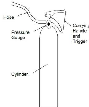
**Components of a portable fire extinguisher: hose, carrying handle and trigger, pressure gauge, and cylinder.**
