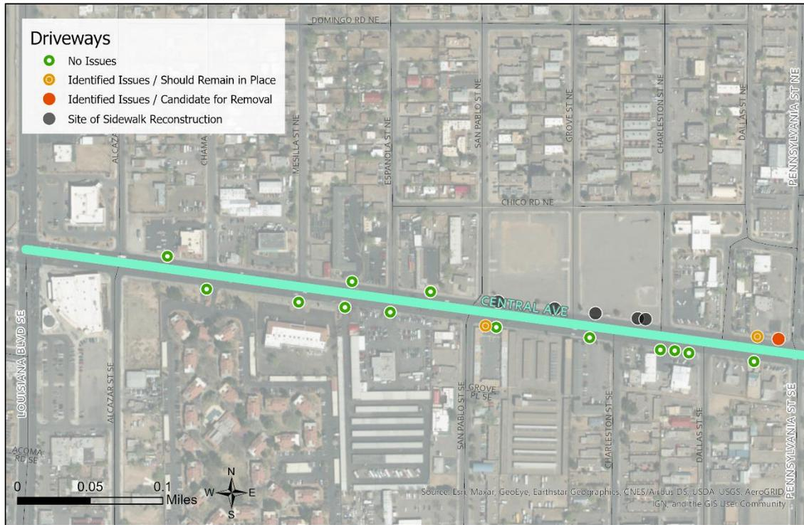
Figure 25: Driveways along Central Ave from Pennsylvania Rd to Wyoming Blvd
