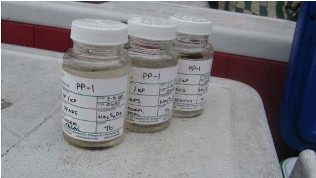
Sample bottles labeled with location, date, time, sample collector, analysis, and preservative type.
