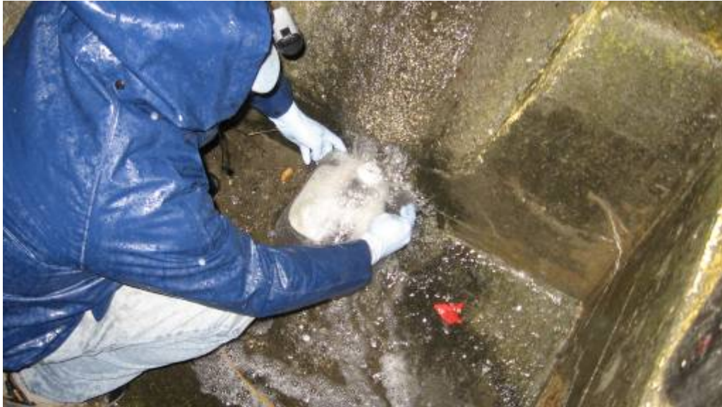
Collecting a sheet flow stormwater sample.
