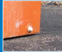
Dumpsters should always have plugs in place.
