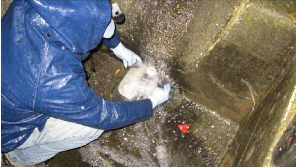
*Collecting a sheet flow stormwater sample.*
