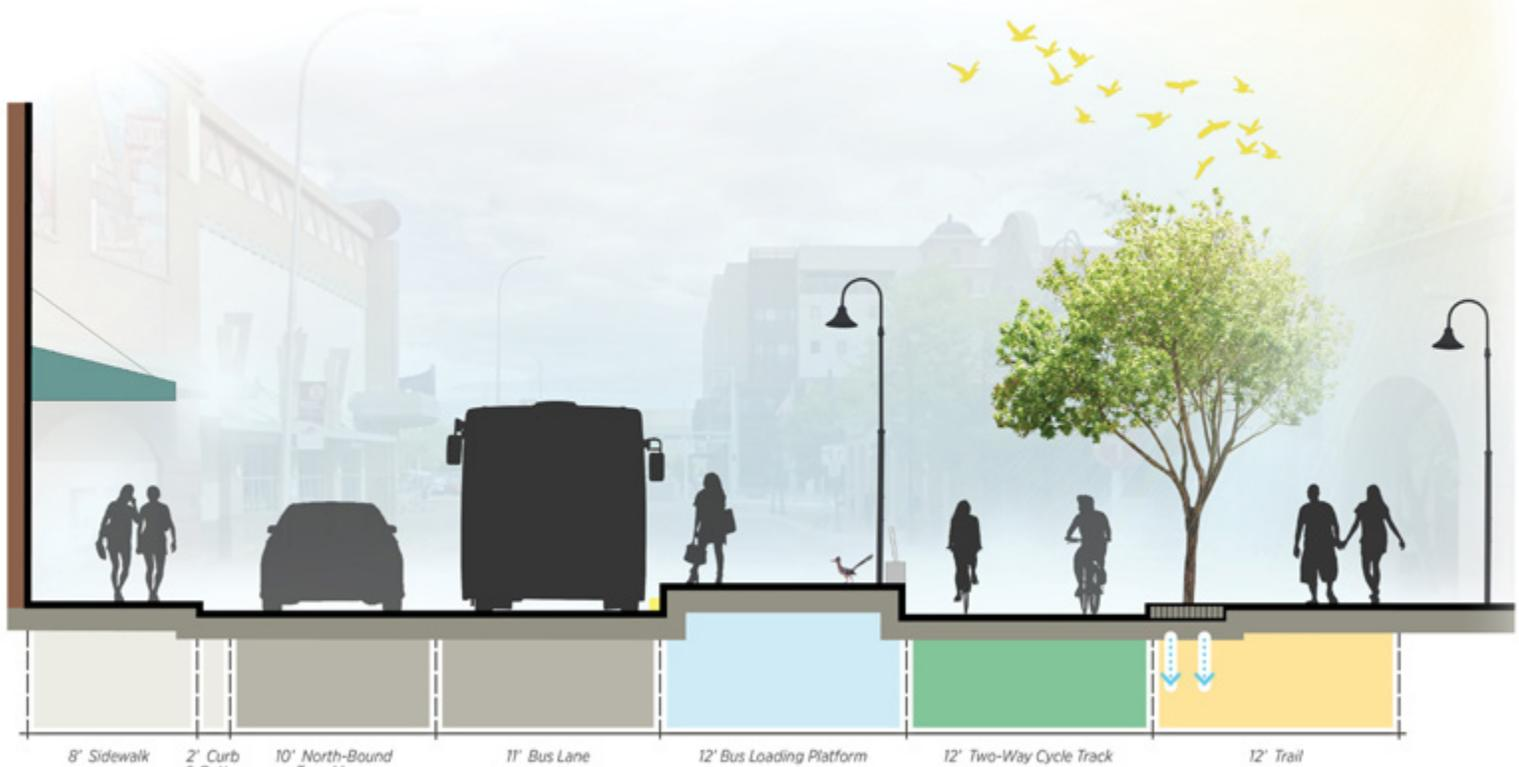
8' Sidewalk    2' Curb & Gutter    10' North-Bound Travel Lane    11' Bus Lane    12' Bus Loading Platform    12' Two-Way Cycle Track    12' Trail
