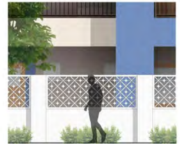
3 Parasoleil Panel (Powder Coated Metal Infill Panel) 3/8" = 1'-0"
