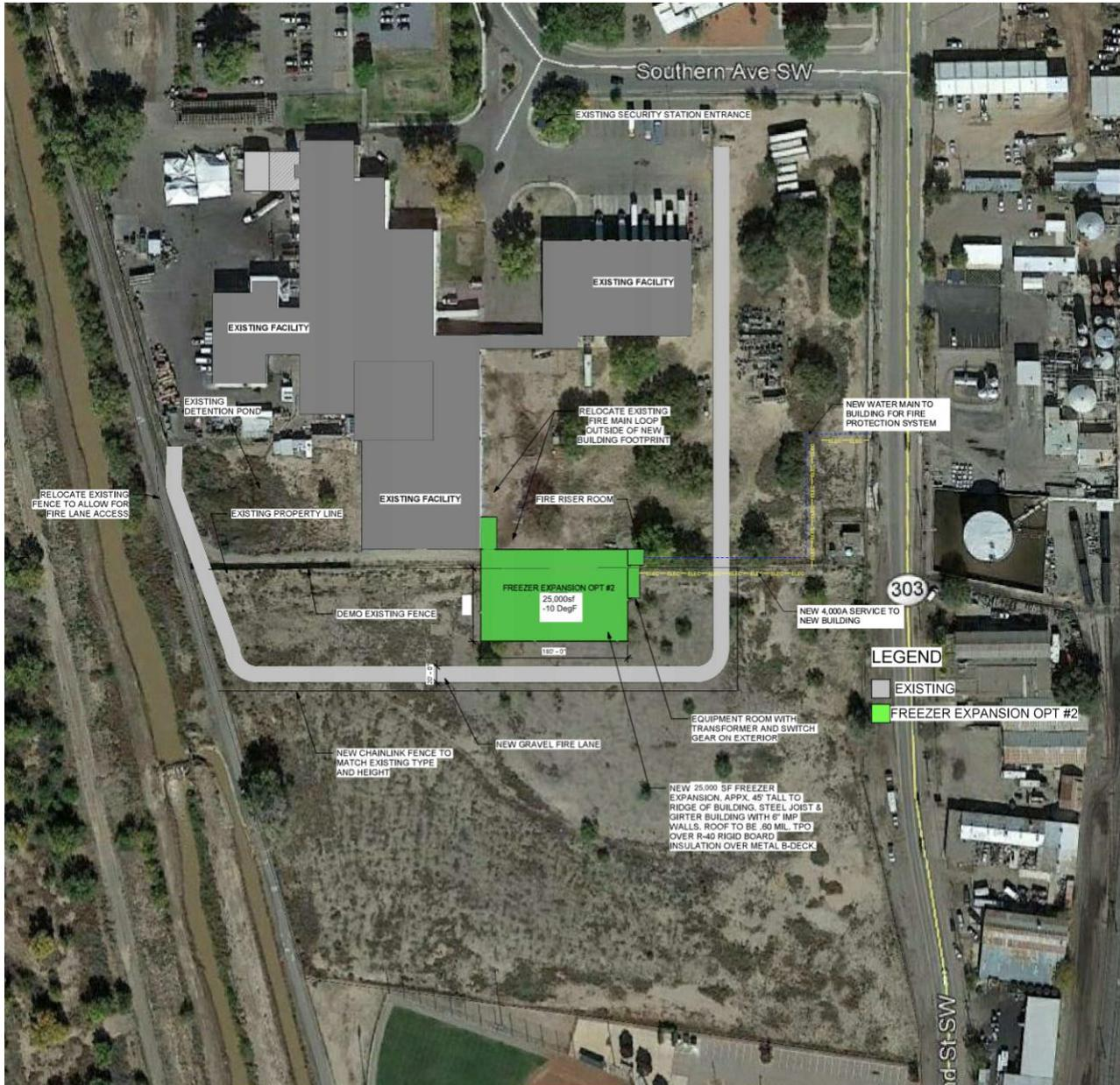
The 25,000-square foot freezer warehouse project involves connection to an existing building. A map of the area is above. Infrastructure, parking, and utilities are already developed. As mentioned, no extension or relocation of utility or road systems is anticipated. There are adequate utilities and roads to the facility.
