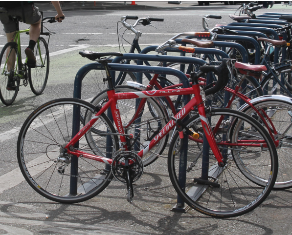
“U” racks allow bicyclists to secure their bicycle at two points and can be configured to maximize bike parking in constrained spaces.
