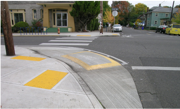
Mountable truck aprons encourage slower vehicle turning speeds while still accommodating larger vehicles.
