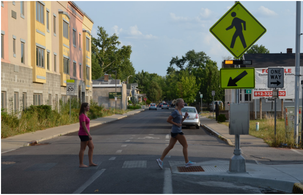
Rapid rectangular flashing beacons (RRFBs) support safe trail crossings at unsignalized and uncontrolled intersections.
