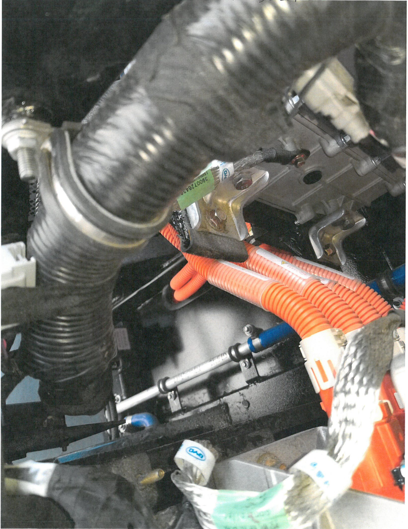
1716- High voltage cables rubbing Frames c13 Engine empty
