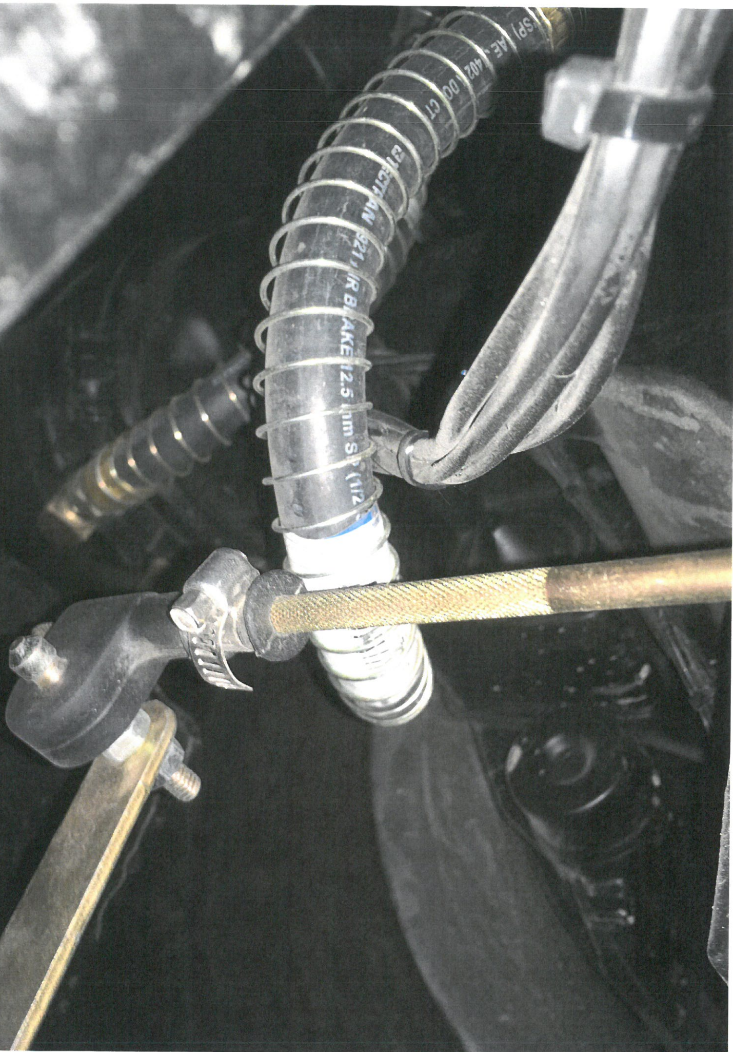
1715 Brake chamber air lines are rubbing
