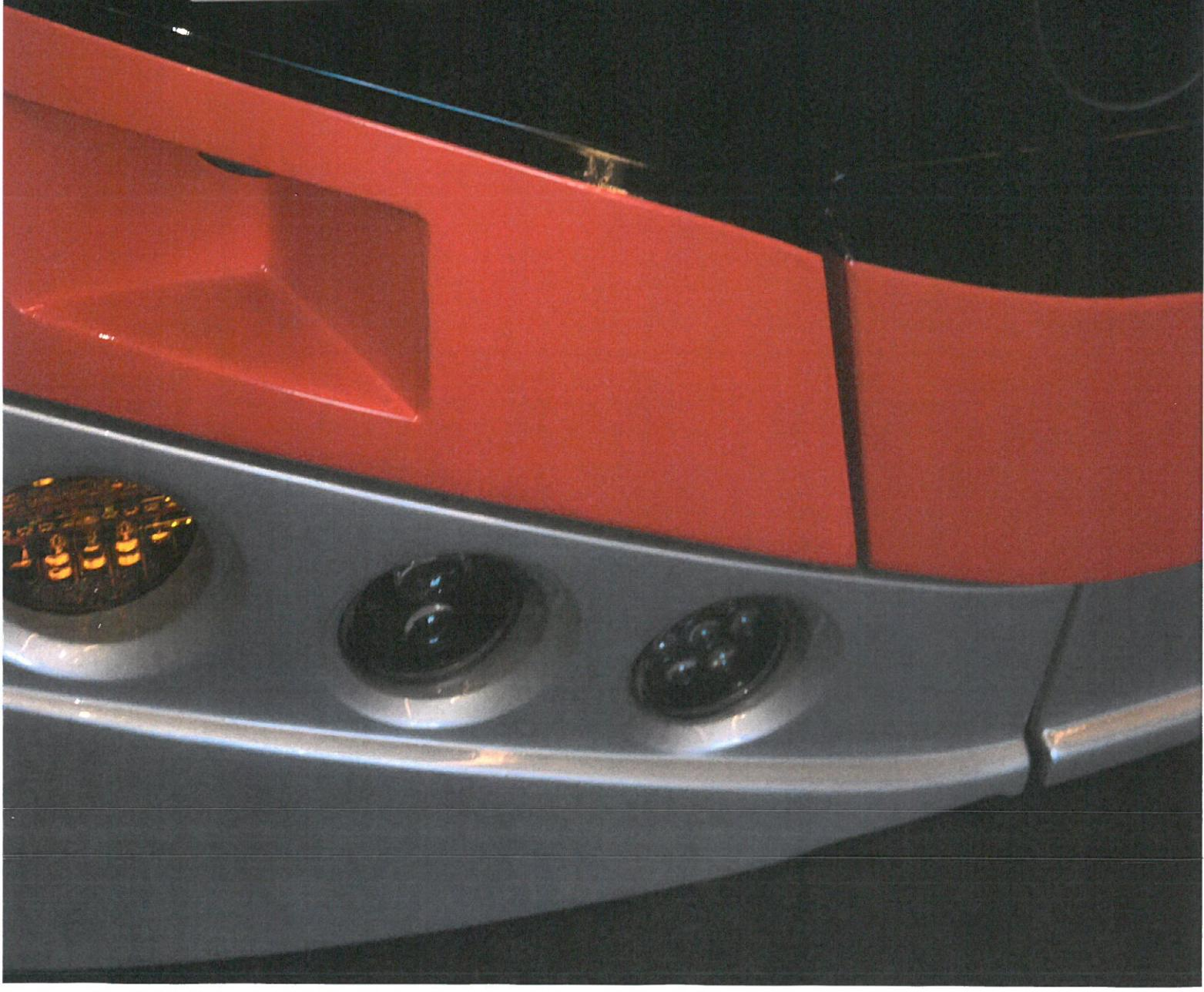
1713 Front of joint, warped panel
