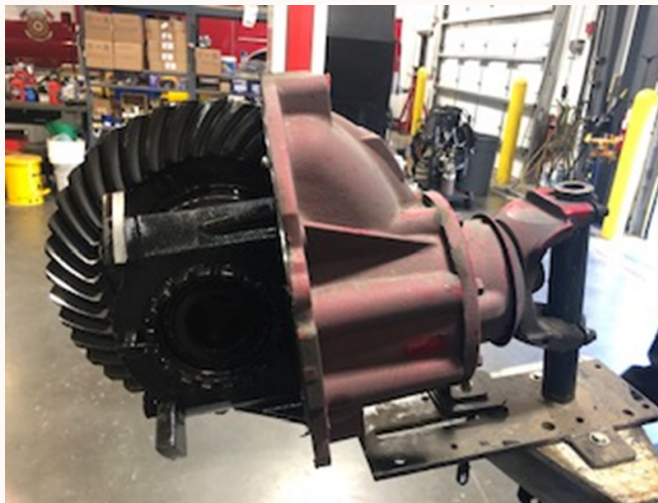
Engine 13 differential replacement.
