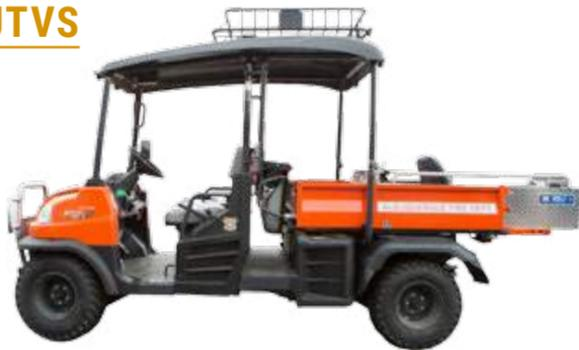
AFD maintains a number of four-wheel-drive, off-road vehicles, called Utility Task Vehicles (UTV), outfitted with gurneys for patient transport. They are the primary EMS vehicle used at high population dense events, or in geographic areas that would be difficult to reach using conventional apparatus – such as at Special Events, the Balloon Fiesta, or in wildland fire applications. They have
