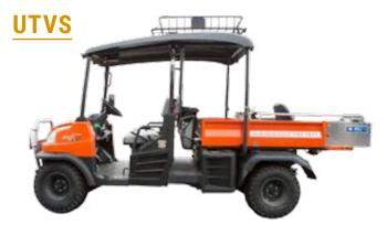
AFD maintains a number of four-wheel-drive, off-road vehicles, called Utility Task Vehicles (UTV), outfitted with gurneys for patient transport. They are the primary EMS vehicle used at high population dense events, or in geographic areas that would be difficult to reach using conventional apparatus – such as at Special Events, the Balloon Fiesta, or in wildland fire applications. They have
