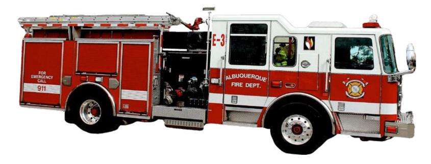
Engine companies – or pumpers – form the core of AFD's emergency response capability. AFD Engines carry hose, and can pump water from their own water tanks. They are housed both in single engine fire stations, as well as at multiple-unit stations, serving with companion ladder truck, light rescues, or Special Operations companies. They are designed primarily for firefighting operations; however, they also are heavily used for EMS, HazMat, auto extrication, and technical rescue.
