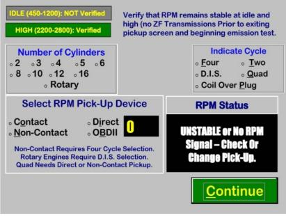
Figures 12 RPM Set-Up Screen
