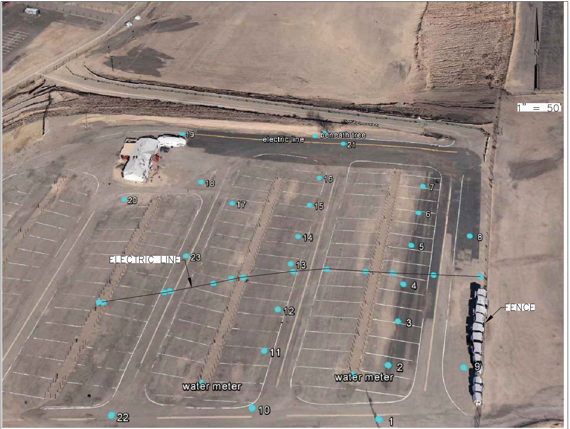
Figure 2 - Gas Probe Locations
