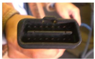
Figure 3 OBDII - Connector
