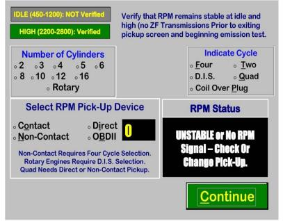
Figures 12 RPM Set-Up Screen
