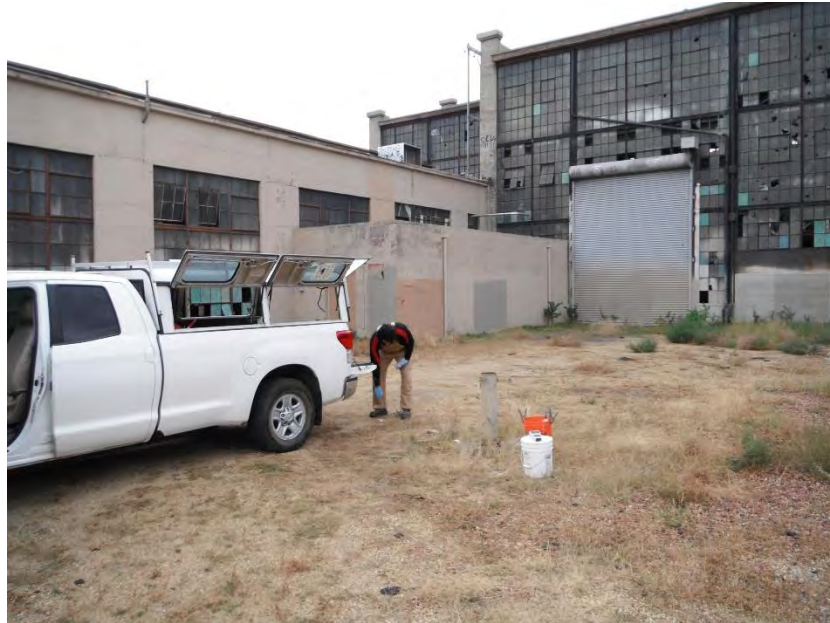
No. 3 – INTERA staff collecting a groundwater sample at monitoring well MW-07.
