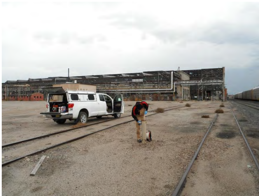
No. 6 – INTERA staff collecting a groundwater sample at monitoring well MW-04.
