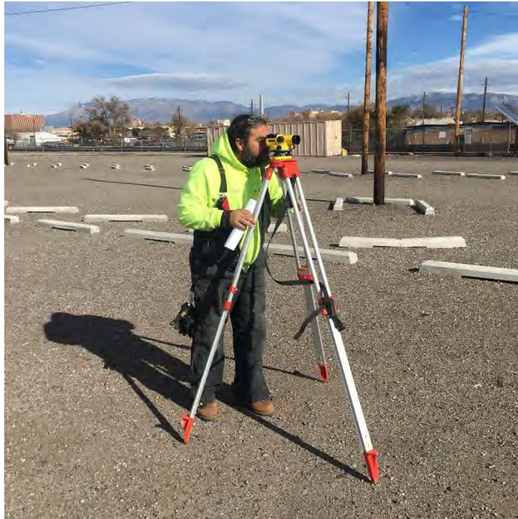
No. 15 – INTERA staff re-surveyed the top of casing elevations for all 8 monitoring wells at the Site.
