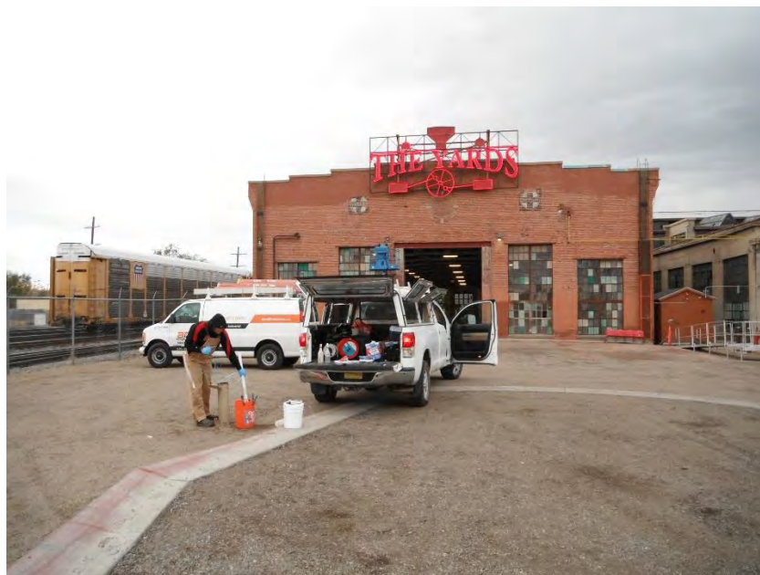
No. 4 – INTERA staff collecting a groundwater sample at monitoring well MW-06.
