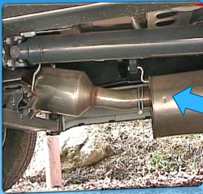
This is a catalyst installed in a modern light truck.
