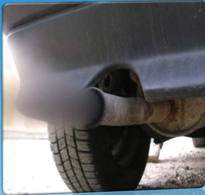
**Diesel vehicle smoke checking: 25% Opacity is OK.**
