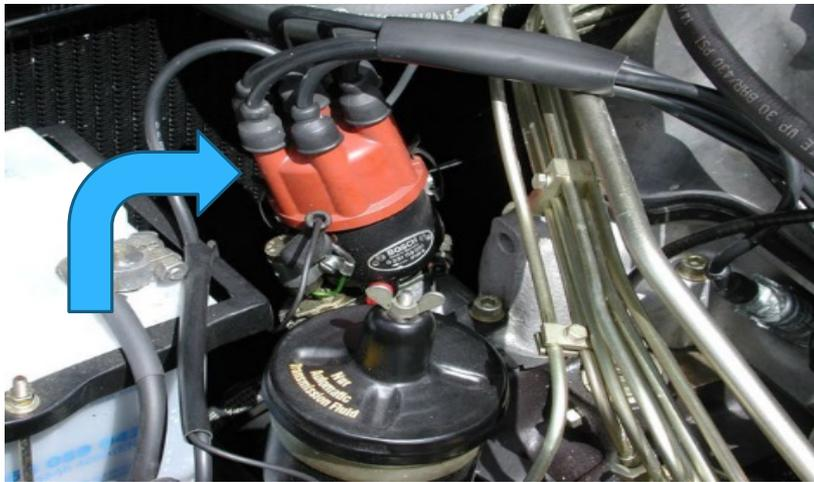
Count the intake plenum runners or spark plug wires can sometimes help to identify number of cylinders.
