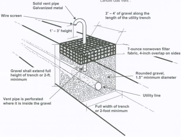
Bottom of vent pipe extends a minimum of 1 foot into the gravel, to the approximate mid-point of the gravel barrier.
