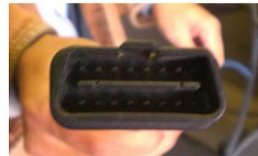
Figure 2 OBDII - Connector
