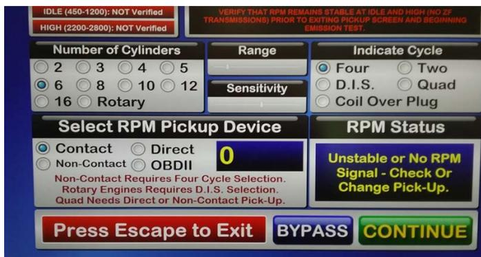
Figure 9 RPM Set-Up Screen
