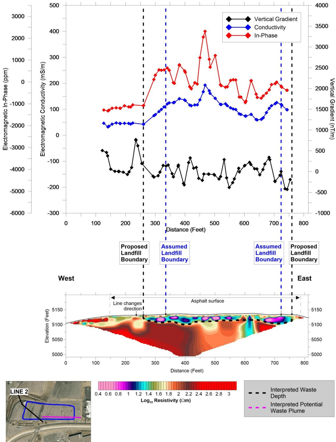
Figure 11. Line 2 Electrical Resistivity Profile.
