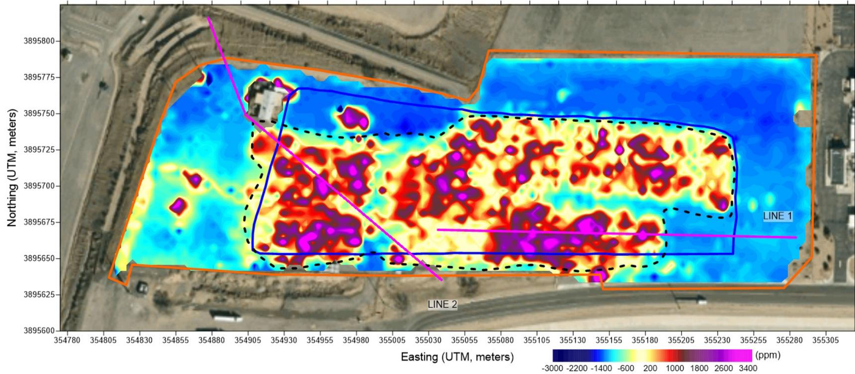
Figure 7. Contoured Electromagnetic Results, Conductivity (mS/m).
