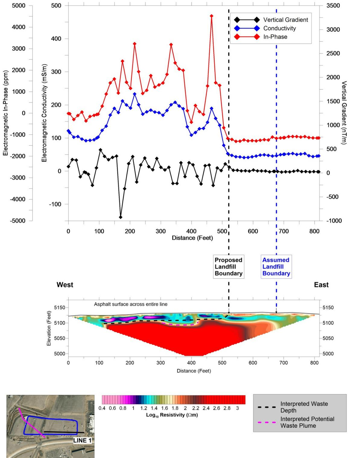
**Figure 9. Line 1 Electrical Resistivity Profile.**
