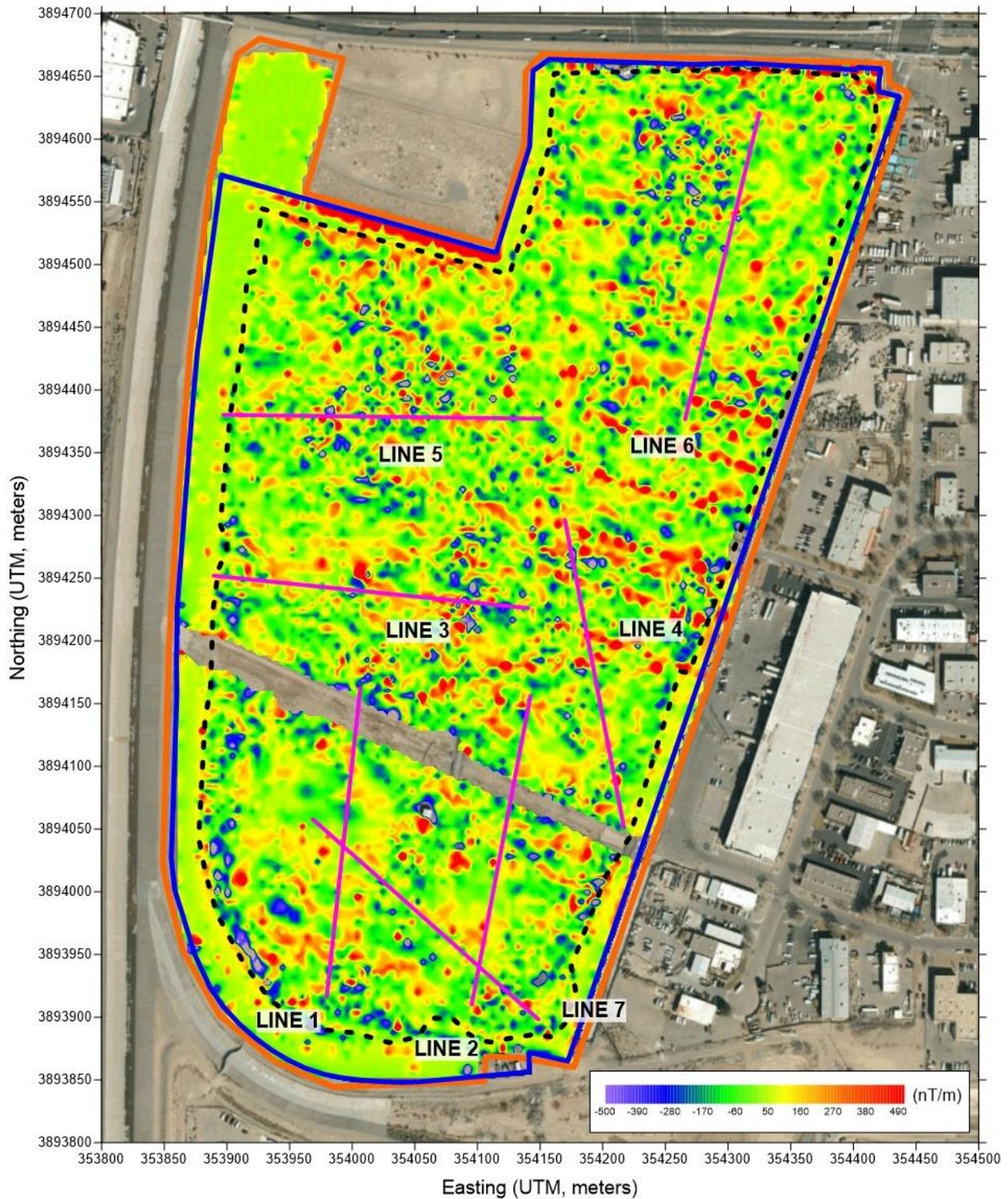
Figure 6. Electromagnetic Conductivity Contour Map
