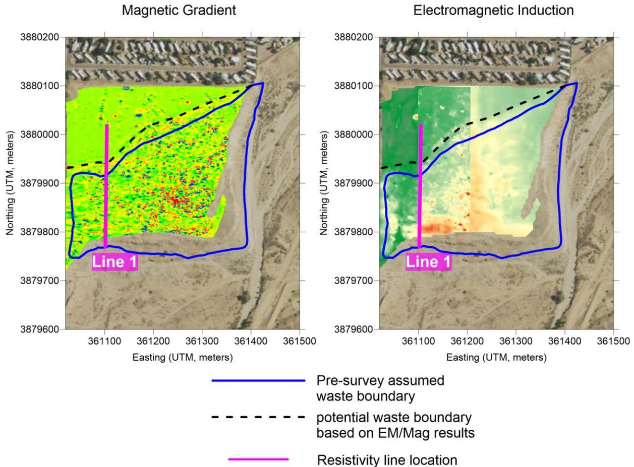
The resistivity data correlate well with the assumed and proposed boundaries as seen in Figure 6. Figure 7 shows the resistivity profile for Line 1 which ran across the NE zone of the survey site, alongside Mag and EM data extracted at the location of the resistivity line. The depth of the waste is estimated at approximately 20 feet, based on the portion of the resistivity profile from 0 to 200 feet, and the thickness of the cover is around 5-7 feet.
