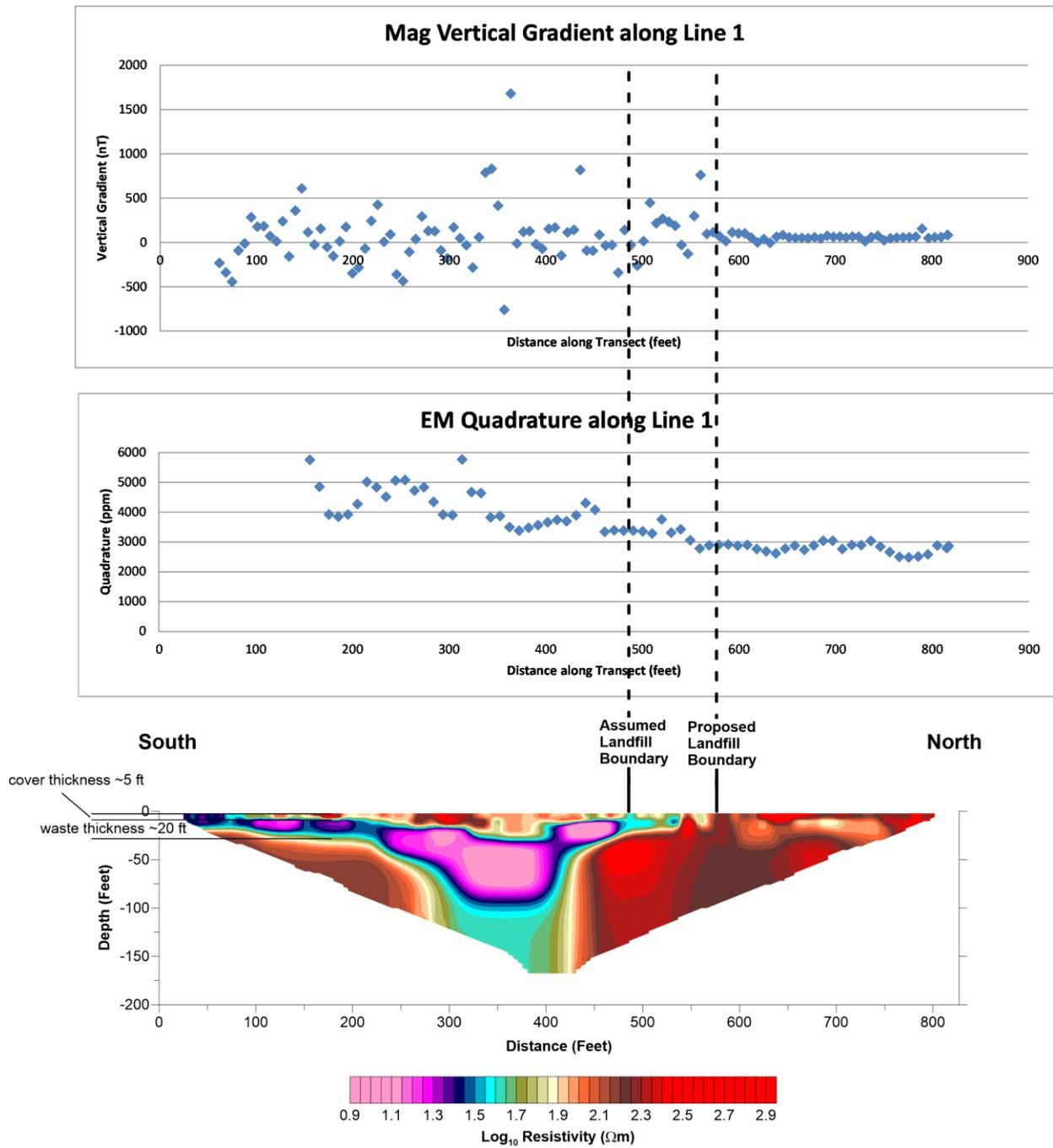
The resistivity data correlate well with the assumed and proposed boundary (same location for this zone) as seen in Figure 8. Figure 9 shows the resistivity profile for Line 2 which ran across the Central zone of the survey site, alongside Mag and EM data extracted at the location of the resistivity line. The depth of the waste is estimated at approximately 25 feet, based on the portion of the resistivity profile from 0 to 250 feet, and the thickness of the cover is around 5-7 feet.
