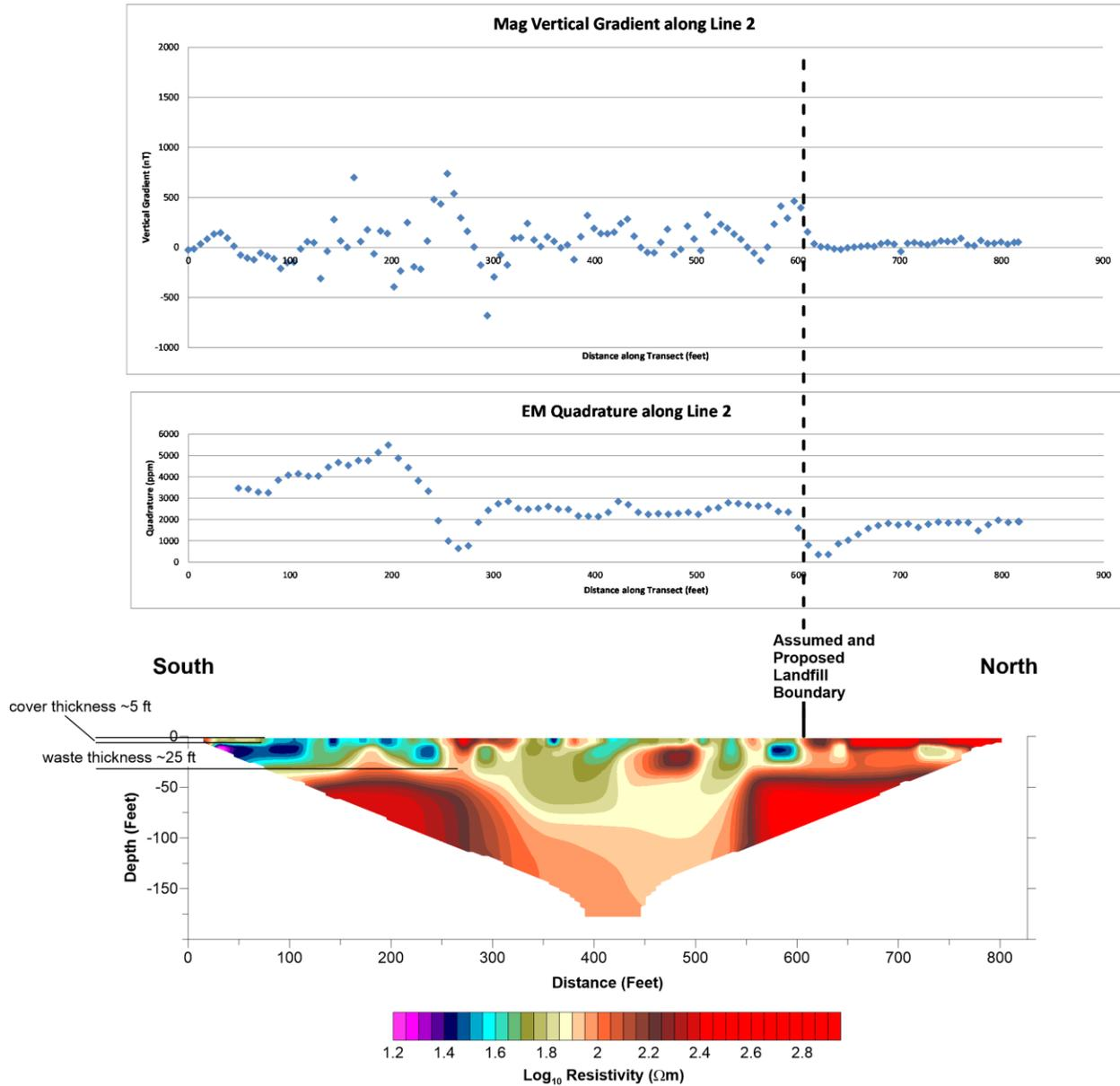
The data for all methods show higher amplitude responses, or higher conductivity, across the first 250 or so feet along the line; this could indicate higher level of waste or moisture in this region of the landfill.
