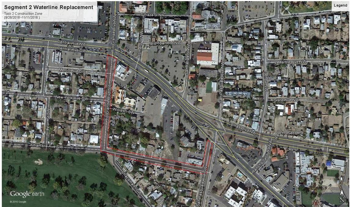
Crews will be installing a new 16" water line that will be replacing a 16" water line that runs from Rio Grande to San Pasqual in Central Ave. The old 16" water line in Central will be grout filled and abandoned in place. As part of this work, an old 6" line
