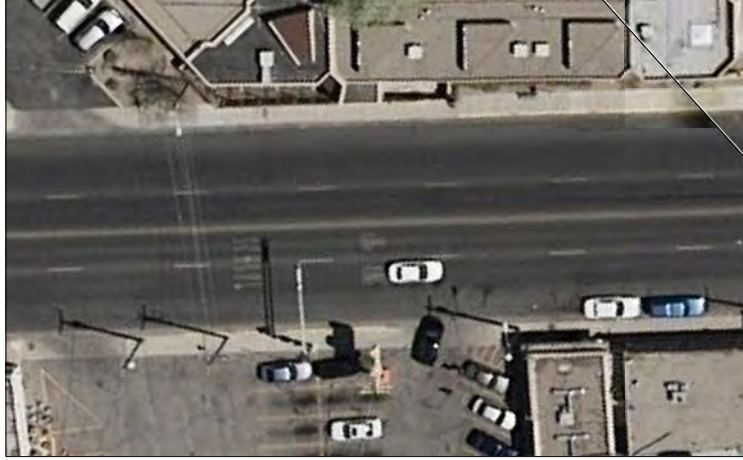
Typical Existing Lane Configuration (Without Left Turn Lanes)
