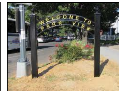
A gateway landmark identifies a unique area or community and indicates a change in environment from a higher speed arterial to a lower speed residential or commercial district
